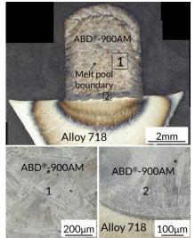
Figure 4: Microstructural assessment of an alloy 718 substrate with LMD ABD®-900AM in as-deposited condition
