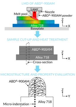
Thin-wall blocks of ABD<sup>®</sup>-900AM were built onto the substrates. A laser spot size of ~1 mm and a bidirectional scanning pattern were used. The length and the width of the build was 80 mm and 4 mm, a build height of up to 70 mm was used, example builds shown in Fig. 3.
