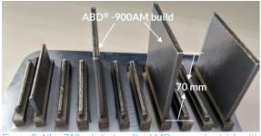
Figure 3: Alloy 718 substrates after LMD processing trials with ABD<sup>®</sup>-900AM.
