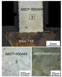
Figure 5: Microstructural assessment of an alloy 718 substrate with LMD ABD®-900AM in heat-treated condition
