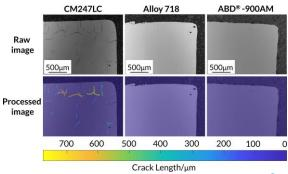
Figure 1: Crack length and distribution maps of CM247LC®, alloy 718 and ABD®-900AM printed by LPBF
